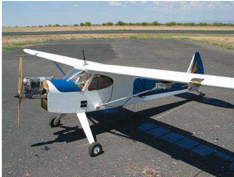
Figure 4.1. SigRascal UAV airframe, with 2.8 meter wing span.
