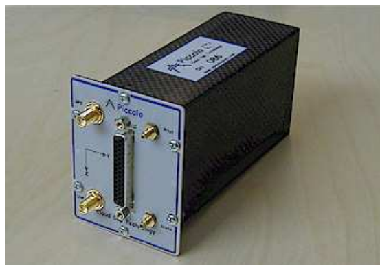
Figure 4.2. Piccolo autopilot system, from CloudCap Technologies. It is 12 cm long and weighs 90 grams.
